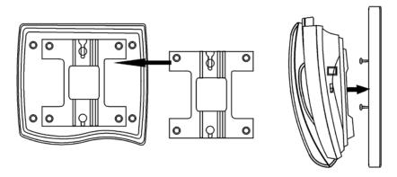
**Note:** If you do not wish to mount your phone on the wall, the Wall Mount Bracket can be reversed to raise the angle of the phone's display when sitting on a table or desk.
